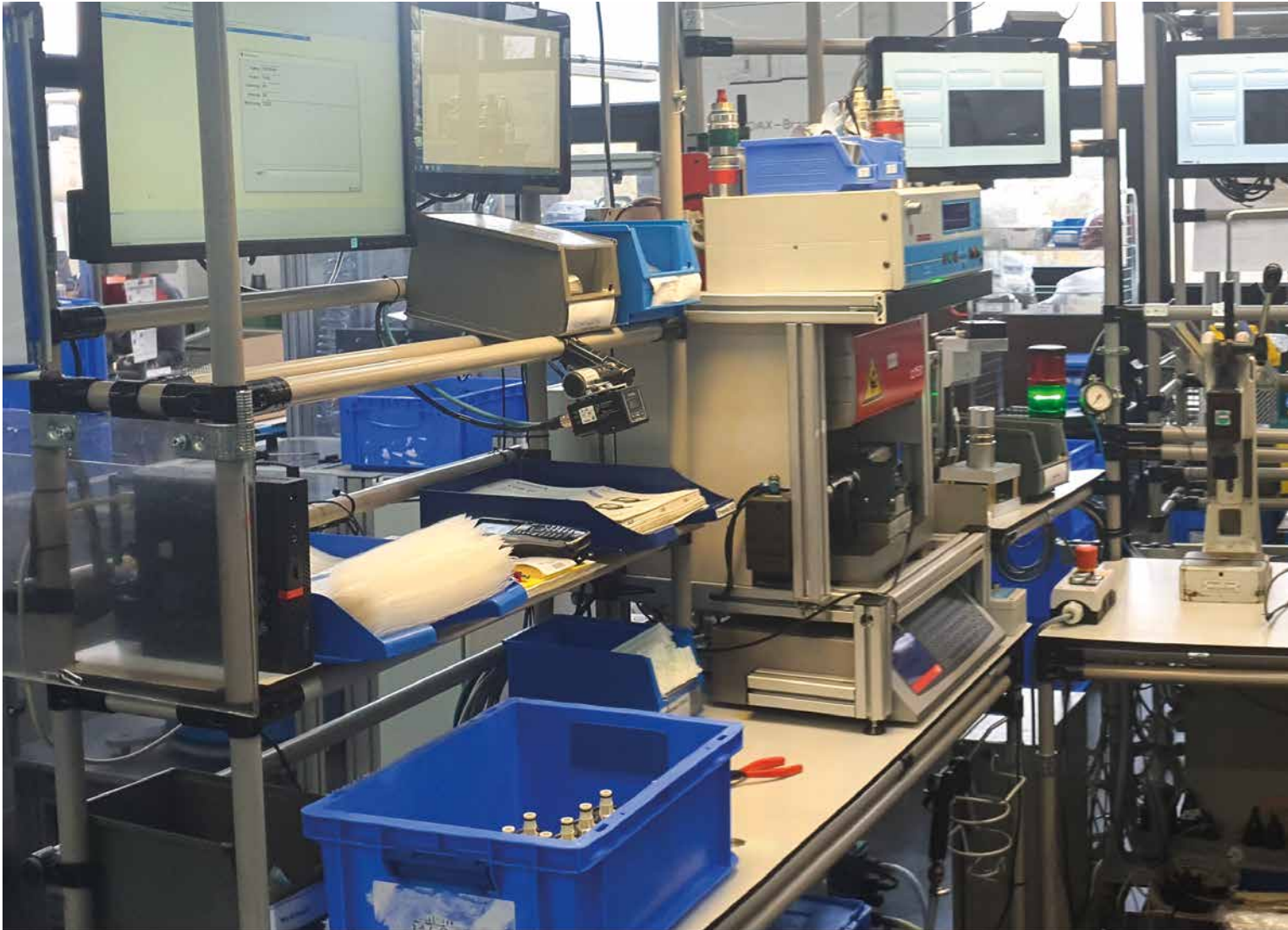
HYDRA Dynamic Manufacturing Control automatically guides the worker through the entire assembly process.
