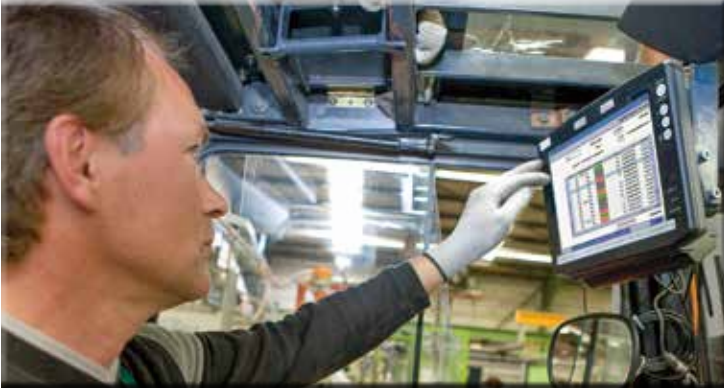
Using a decentralized transport management in MES HYDRA, the forklift driver can decide which available transport order is produced. Therefore central transport planning is omitted.
