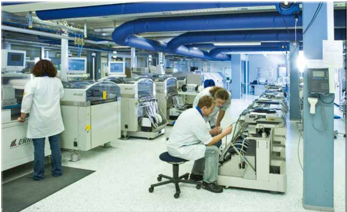
A total of three SMD lines produce a high volume of data at HEKATRON. 300 million components are installed onto 3 million flat modules annually.
