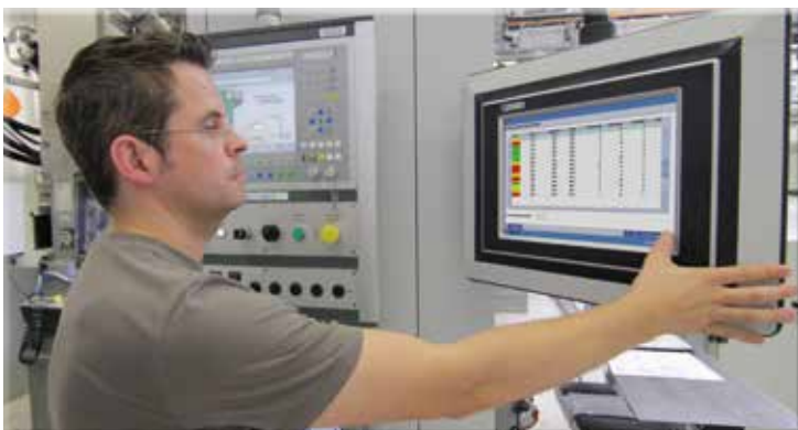
The operator is instantly informed on the electronic Kanban board in MES HYDRA about the status of each cycle. Central intervention is not needed.
