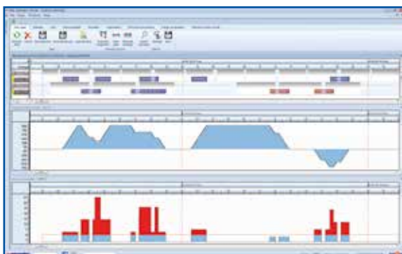
Material stock development (chart in the middle) and the forecasted energy consumption (bottom chart) can be displayed in the HYDRA Shop Floor Scheduling.
